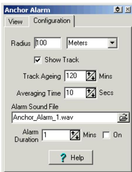
**Radius** - The radius from the anchor position. if the vessel leaves this circle the alarm will sound.
