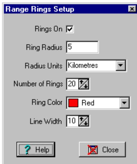
**Rings On** - When checked the rings are drawn around the GPS position.
