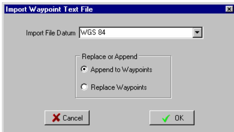
The datum used for importing (the datum used for the positions in the file) can be specified, if the datum is in the file in one of OziExplorers standard datums then it will default to this.
