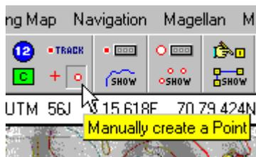
Press the Manually Create Point button on the Toolbar. Click on the map to create a point. The Point Control can be used to modify the behaviour of point creation.
