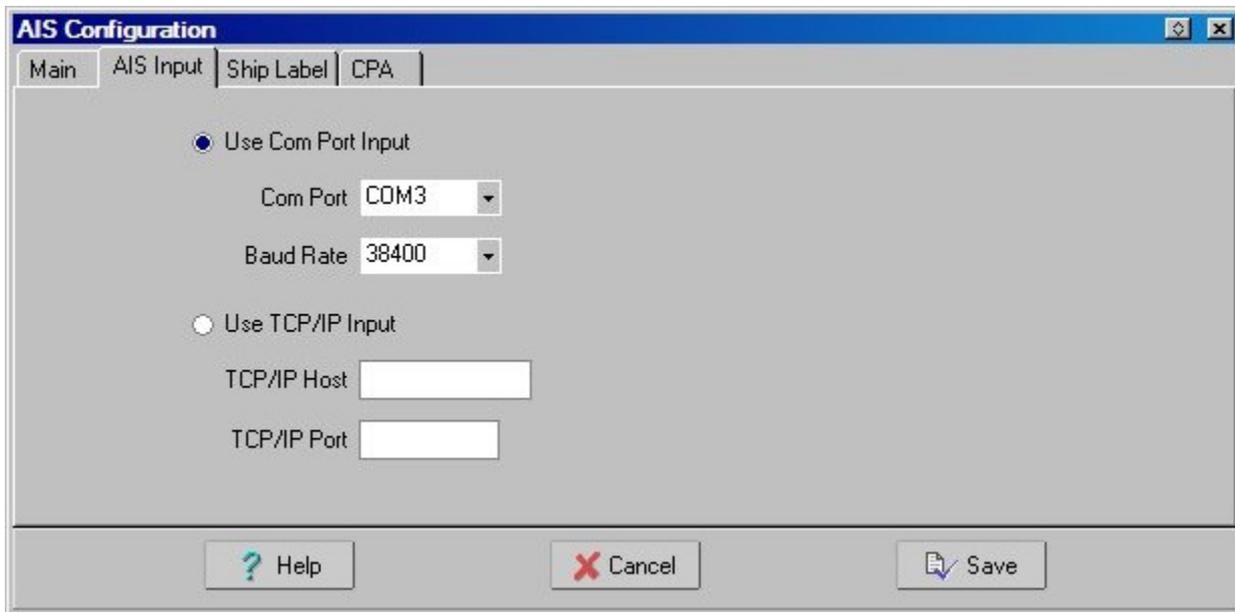
**Use Com Port Input** - If you have a AIS receiver connected to a com (serial) port.
