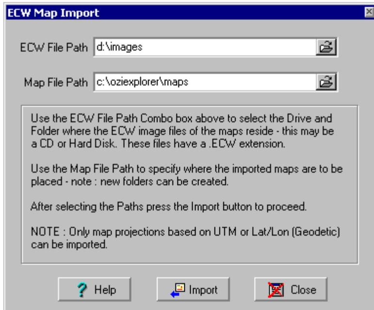
**Image File Path** - The Path where the ECW image files are located.
