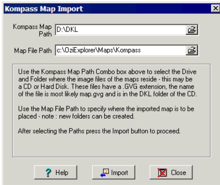
**Kompass Map Path** - The Path where the Kompass map is located, the map file is most likely map.gvg and is in the DKL folder on the CD.
