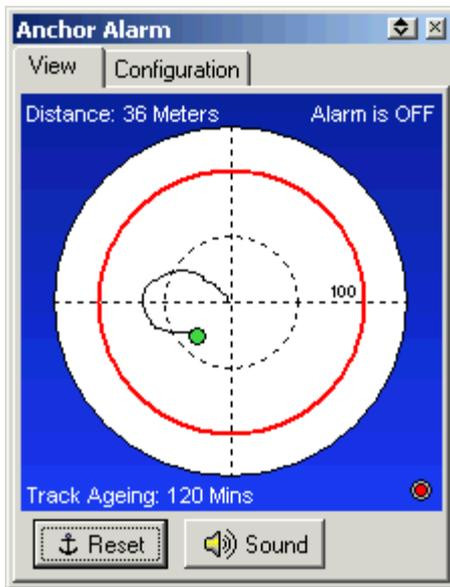
The center of the circle is the vessels anchor position.
