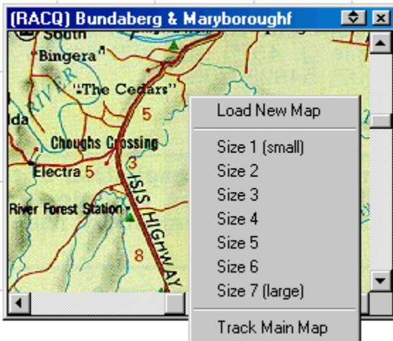
The regional map window is used when using moving map (real time tracking) mode, it shows your position on a map loaded in the regional map window. When not using moving map mode it centers on the center of the main map.
